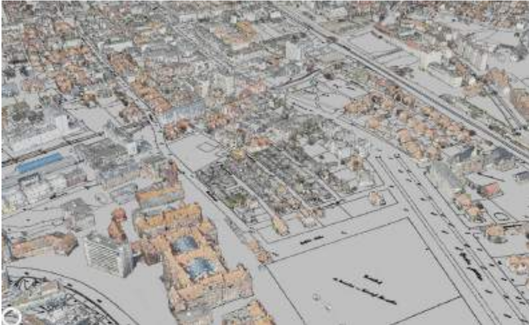
Fig. 233. Filtered aerial lidar point cloud of Gdańsk University of Technology, projected to the map of 1930 in ArcGIS. Source: author.
