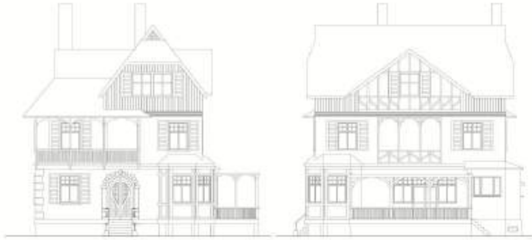
Fig. 200. Elevations of digitally reconstructed model of officers’ villa, synthesis of knowledge. Source: author.
