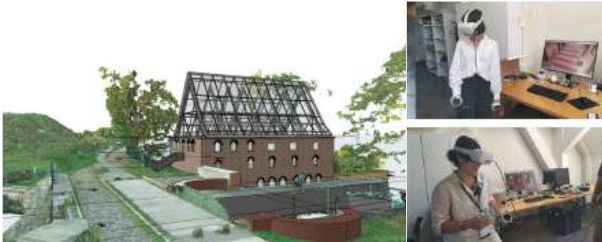
Fig. 162. Adaptive reuse concept design. Visualisations of exterior and interior of adapted watermill showing the potential conceptual design using BIM software with TLS laser scan integration. Source: Silvia La Placa, Andrea Bongini and author.
