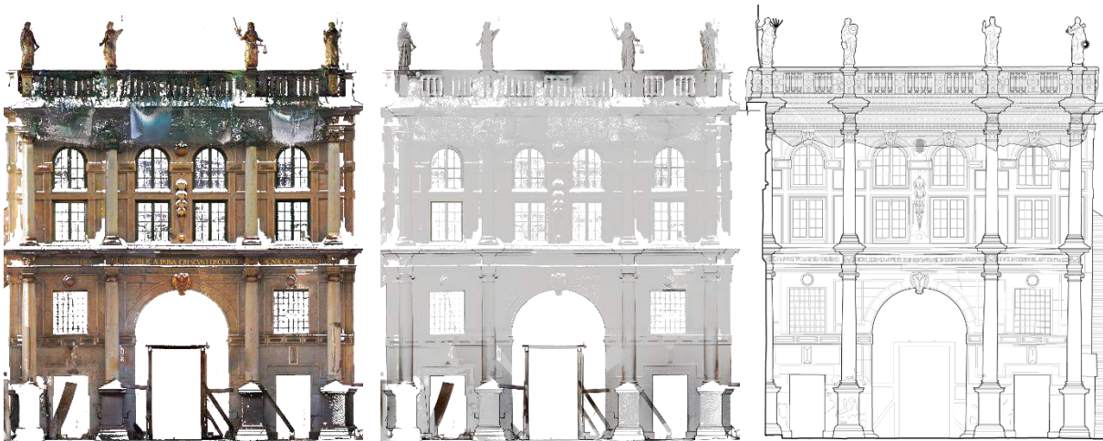
Fig. 151. The Golden Gate in Gdańsk. Left: laser scan orthophoto; centre: laser scan orthophoto with adjusted opacity; right: synthesised inventory drawing derived from the digital survey. Source: author, drawing by Zofia Piwońska.
