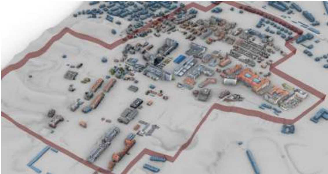
Fig. 238. Simplified model showing 2025 using segmented building from a scanned photogrammetry model with integration of TIN buildings and a mesh terrain model. Source: author.
