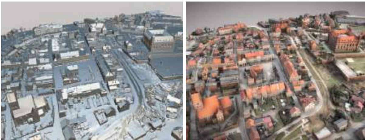
Fig. 146. Urban scale photogrammetry: Comparison of untextured mesh with textured mesh of historical city centre of Gniew in Metashape software. Source: author in cooperation with Paulina Bone 788 .
