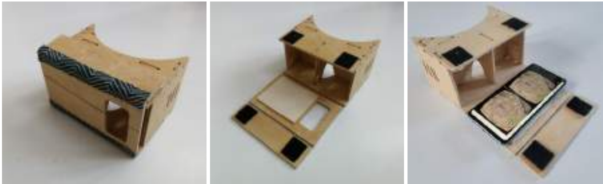
Fig. 153. VR phone holder with spherical lenses, made of plywood and based on the original Google Cardboard design. Designed by Szymon Kowalski and cut on a CNC machine 791 . Source: author.
