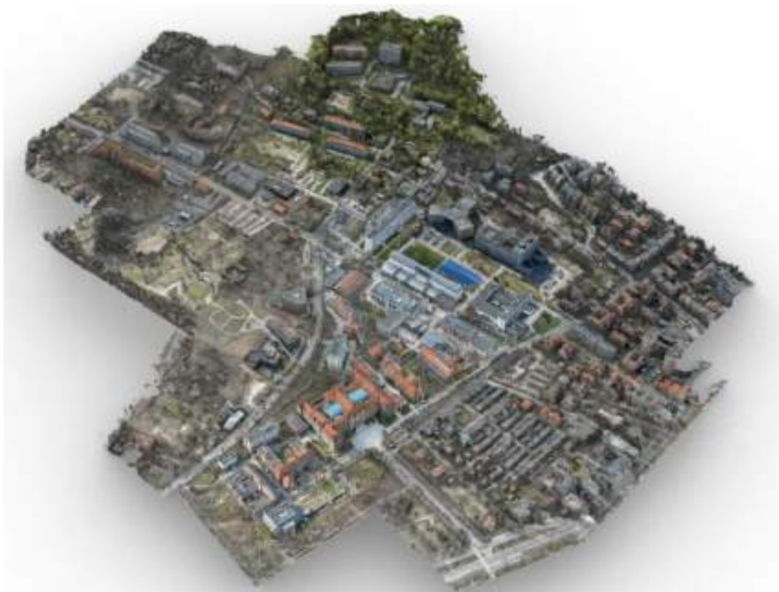
Fig. 237. The six individual aerial photogrammetry scans of the entire area were joined and unified into a single master scan. Source: author.
