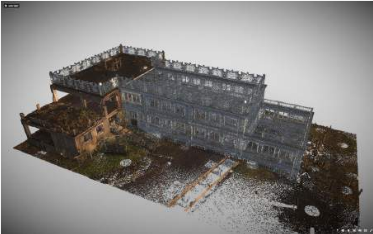
Fig. 214. Partial Digital Reconstruction of the missing wing of New Barracks, using the point cloud solution adjoined to the original scan, based on the architectural investigations 952 . Source: author in collaboration with Wojciech Samól.
