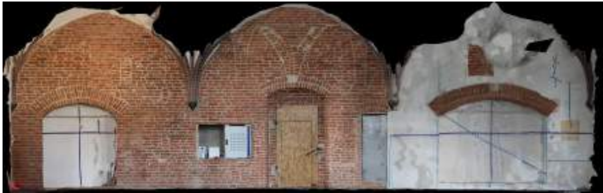
Fig. 171. Digitized elevation of the northern wall of the sacristy, with blue markers introduced to correct distortion during photogrammetry scanning. Source: author.
