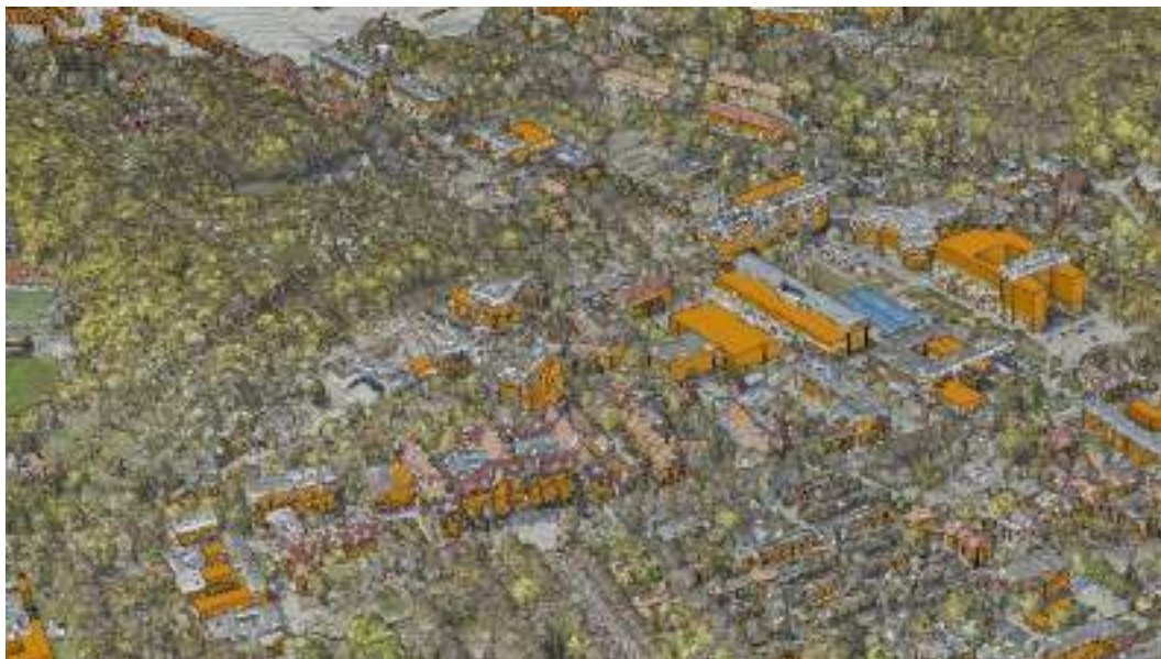
Fig. 232. Aerial Lidar point cloud of Gdańsk University of Technology and area of Heiligenbrunn in ArcGIS software. Source: author.
