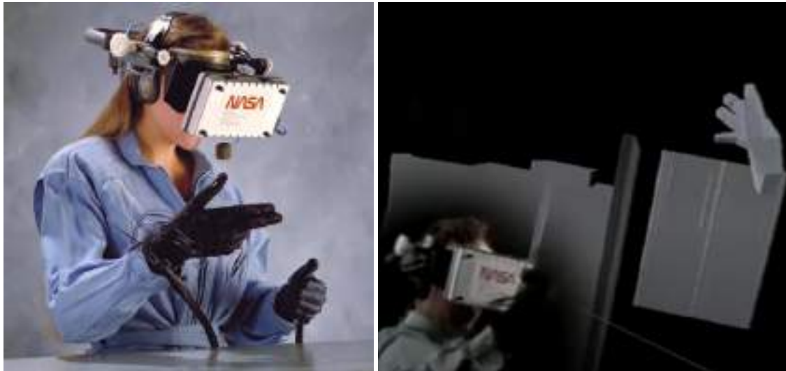
Fig. 109. Left: Nasa's VIEW with Head Mounted Display and use of wired glove controller. Right: VIEW system graphic environment with virtual hand, based on wired glove controller, (source: Association for Computing Machinery 680 ).
