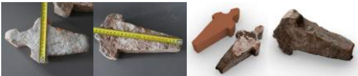
Fig. 172. Brick measurement for photogrammetry scaling and digitized Gothic rib profile bricks. Source: author.
