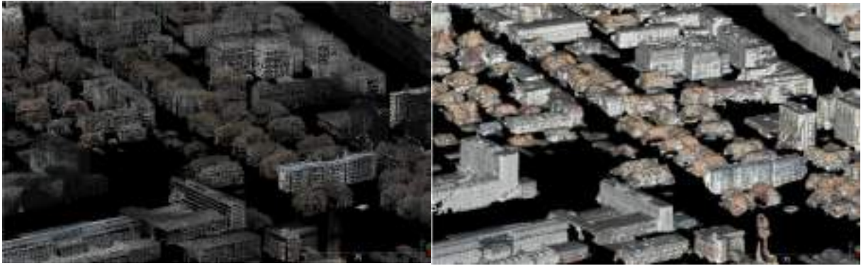
Fig. 235. Left: filtered aerial lidar point cloud of the Wrzeszcz district acquired via Geoportal and processed in ArcGIS. Right: the same point cloud transferred into the mesh model. Source: author.
